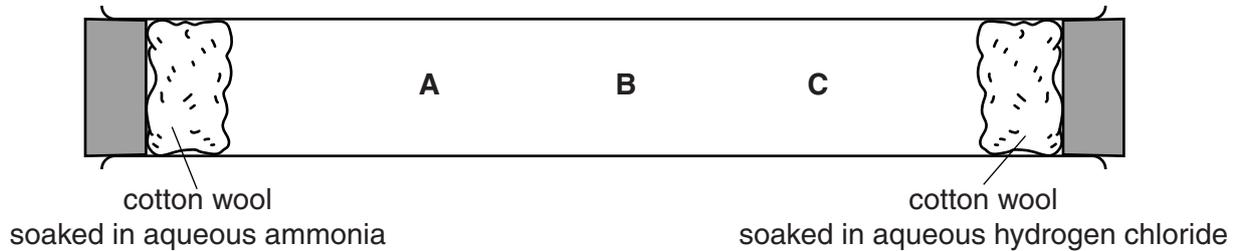
After a few minutes, a white solid is produced on the inside of the tube.
