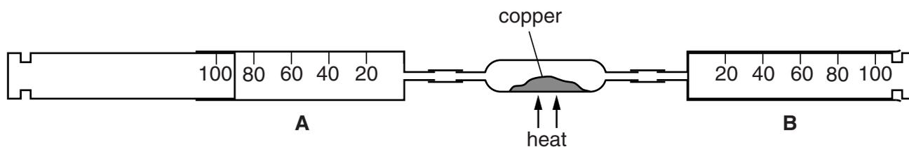
Syringe **A** contains  $90\text{cm}^3$  of air. The air is forced over heated copper into syringe **B**. The air is then forced back over the heated copper into syringe **A**.
